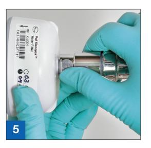
Pall Kleenpak In-Line Disposable Water Filters (KAQIN) may be used for up to 31 days. To remove the filter, push the thumb latch each connector adaptor to release.
